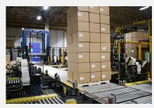
STACKED PALLETS DISCHARGE FROM EACH BOX BOT CELL BUILD STATION ONTO A CENTRALIZED TRUNK LINE THAT CONVEYS TO AN AUTOMATIC STRETCH WRAPPER.
