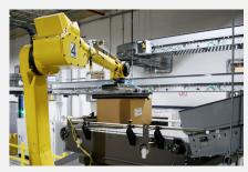
ACTIVATED ROLLER BELT (ARB) CONVEYORS ENSURE CASES ARE REGISTERED TO THE CORRECT LOCATION PRIOR TO PICKING WITHOUT THE USE OF CLAMPS OR OTHER DEVICES.
