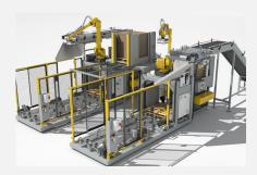
16 SKID-BASED BOX BOT SERIES PALLETIZERS WITH 6-AXIS ROBOTS ALLOW FOR ROBOTIC PLACEMENT OF PALLETS AND SLIP-SHEETS WITHOUT THE NEED FOR ADDITIONAL FUNCTIONALITY ON THE ROBOT'S EOAT.
