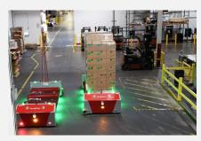
THE IAVS SAFELY MANEUVER ALONGSIDE OTHER WORKERS, CONTROLLED BY INDUSTRY LEADING SAFETY FIELDS THAT INSTRUCT THE VEHICLES TO START, SPEED UP, SLOW DOWN OR STOP WITH NO NEED FOR ANY MAGNETIC TAPE OR OTHER PHYSICAL GUIDES.
