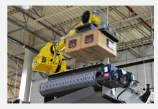
A VENTURI VACUUM GRIPPER END-OF-ARM-TOOL WITH FOAM PAD HANDLES CORRUGATE CASES, SLIP SHEET AND PALLETS.
